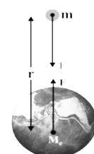
Figure 5.2: Weight of a body is due to the gravitational force between the body and the Earth.
